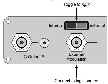
External Modulation is logic-level controlled. A logic HI on External Modulation will select the "straight-thru" amplitude configuration; a logic LO will select the "crossed" amplitude configuration. The setting of the front-panel amplitude crossover switch will be ignored. As with Internal Modulation mode, adjustments may be made to either amplitude as the controller toggles between them.
