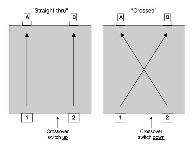
In the "straight-thru" configuration, LC output A is controlled by the amplitude 1 knob, and LC output B is controlled by the amplitude 2 knob. In manual mode, the "straight-thru" configuration is selected by setting the front-panel crossover switch up.
