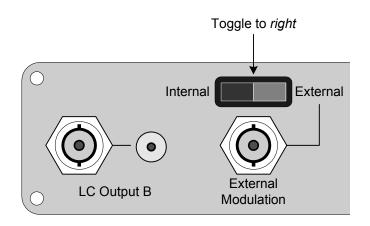
modulation source attached to the External Modulation connector, this will enable manual mode.
