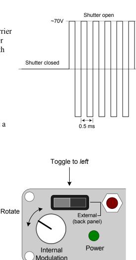
It is possible to route the Internal Modulation frequency to the back-panel BNC connector as a driver output for synchronization purposes. Contact Optical Finesse for further details.
