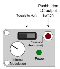
When the high-voltage output is enabled, it is normal for the driver to emit a quiet, highpitched humming sound.
