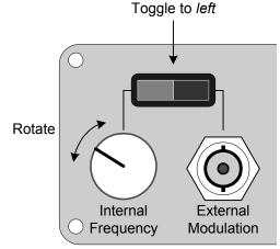
As the controller toggles, the RMS voltmeter reading will alternate between the two preset amplitudes. For faster modulations, the meter will be unable to keep up with the actual LC output, and will display an intermediate value. This is normal controller behavior. If an accurate reading is desired for either or both presets, switch the backpanel toggle switch to the External setting to return to manual toggle mode.
